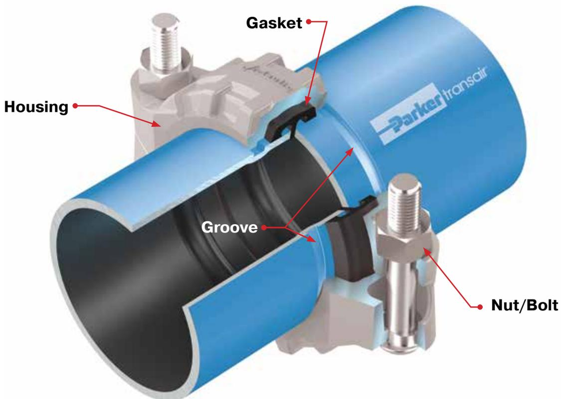
8" pipe to pipe connectors can be quickly connected to Transair pipe. Position the seal on one half of the pipe, then slide the 2nd pipe into position. Lastly, attach the connector over the seal and tighten.
