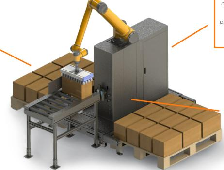
The included frame and chassis acts as a housing to store the cables. mechanics, and the control box out of view. The Palletizing Station is a turnkey solution that moves as one piece without the need for any internal configuration or wiring; minimizing downtime by making deployment and initial setup a breeze.
