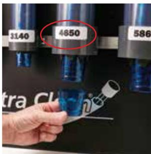
Capsule identifier (size, part number) labels provided for dispenser tubes for easy identification, loading and re-ordering.
