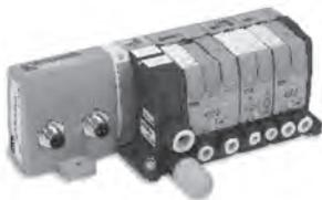
The P2M IO-Link Class A module can handle a Moduflex valve manifold having up to 19 solenoid outputs, or H Series Micro / ISO up to 24 solenoid outputs.
