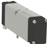
A single solenoid HA valve mounts on top of the PXM pilot exhaust module. It is the first valve and works in conjunction with the PXM to control pilot across other valves in the manifold.
