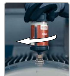
Screw lubrication system into lubrication point
