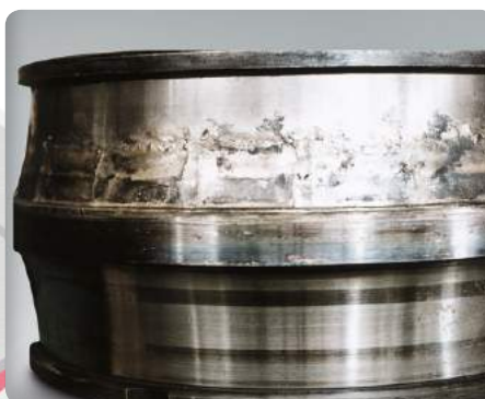
Bearing damage caused by lubrication starvation
