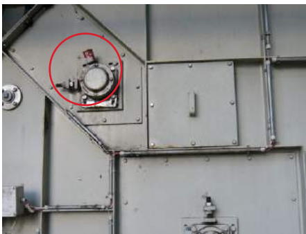
Lubrication of flange bearing on bucket conveyor
