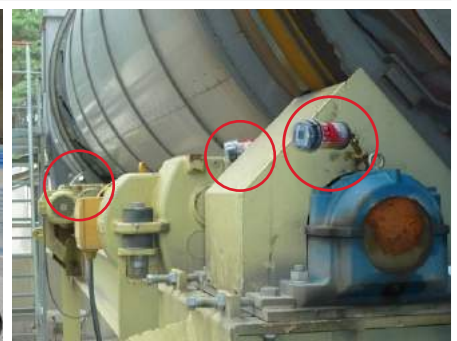
Lubrication of pillow block bearing on rotary dryer
