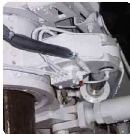
Quicklub divider valve mounted on a milling machine
