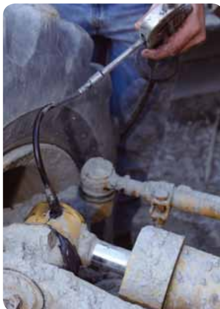
When manually lubricating a bearing, grease is not typically evenly spread inside the bushing and not completely purged
