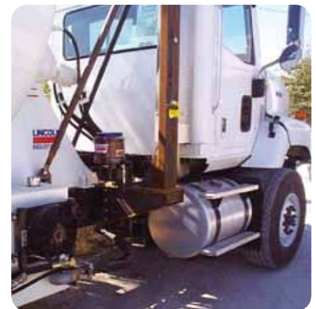
Quicklub system installed on a ready mix truck
