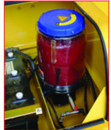
Quicklub® 203 Pump Eight-liter, 24 VDC pump with integrated timer, low level and system alarms
