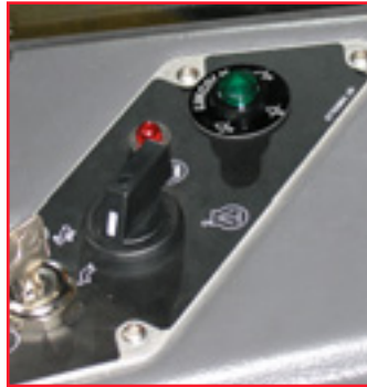
The optional warning light alerts the operator if the pump reservoir is low or if a lubricant line is blocked. This also functions as a manual button to initiate a lube cycle
