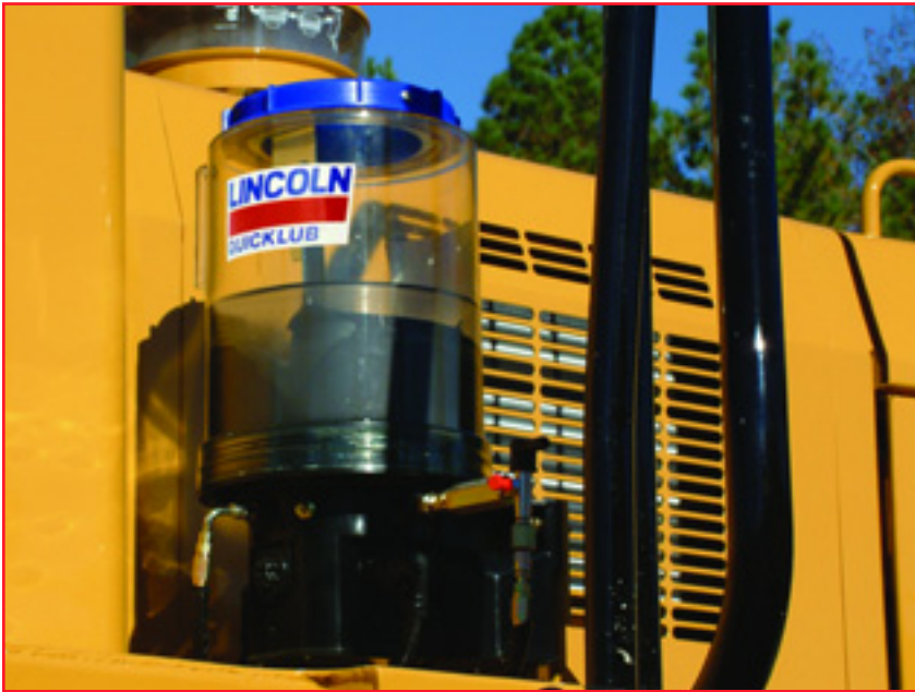
Typical Quicklub® pump mounted on operator deck behind the cab for ease of visual monitoring and service
