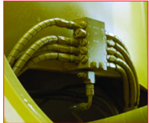
Quicklub® metering valves ensure more grease is delivered to high-demand bearings
