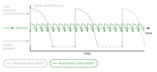
Manual lubrication typical results in over-or-under lubricating. Automatic lubrication delivers a consistent amount for optimal machine performance.
