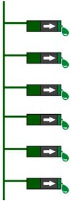
A single line parallel system can service a single machine, different zones on a single machine or even several separate machines and is ideal when the volume of lubricant varies for each point.
