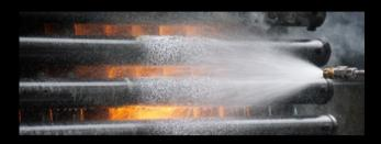
Providing exceptional cooling abilities and Class A (debris) and Class B (fuel) fire suppression, customers around the world are adding **AFEX** liquid agent systems to their fire protection programs. The **AFEX** liquid agent works by cooling hot surfaces, separating fuel hydrocarbon molecules to prevent it from igniting, and forming a layer of foam to suffocate the flame. The liquid agent is suitable for temperatures as low as -40°F (-40°C).
