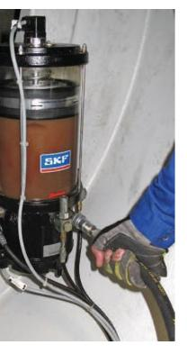
of grease to be dispensed during each lubrication maintenance session. even though SKF WindLub lubrication systems require minimal maintenance. lubricant must be reilled from time to time. Tower heights and tight working spaces create unique challenges for maintenance workers.
