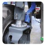
Grape harvester components are exposed to high-vibration loads and need reliable lubrication every day they are used. SKF ProFlex and Lincoln Quicklub automatic lubrication systems help free up time for other wine-making tasks. Singlepoint, automatic lubricators also are well-suited for these machines.
