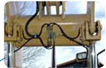
Metering devices correctly positioned out of harm's way and properly anchored to stay that way
