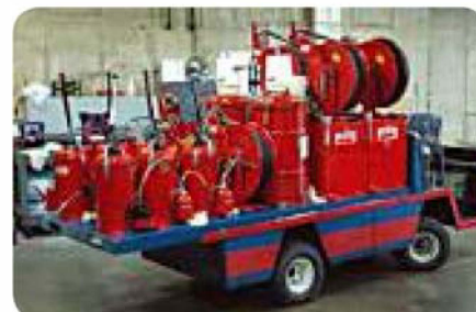
In-plant lubrication trucks take all the important fluid lubricants to the machinery. This electric cart even includes a waste oil evacuation system.
