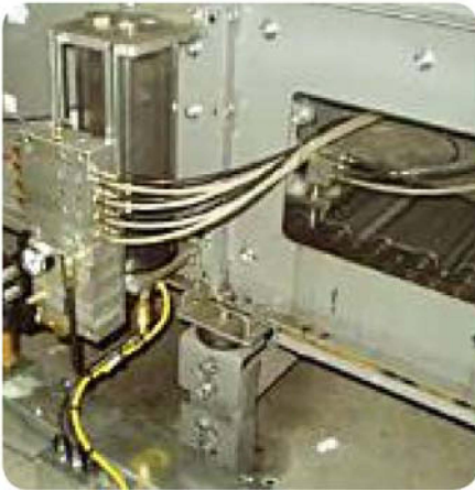
An Orsco VSR system lubricates a conveyor chain on an oven application in a food plant.
