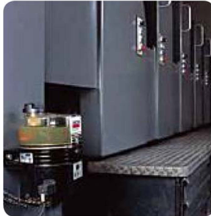
This Lincoln Quickclub QLS oil system virtually eliminates manual lubrication on bearings and gears for this printing press. Lubricating on-the-fly improves productivity.
