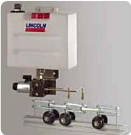
The PMA solenoid pump is designed for contact-free oil lubrication of the chain. The exact metered amount of oil is applied to the chain pins only.
