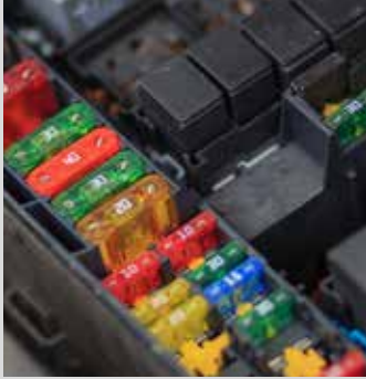
Inspection of car fuses – color and material
