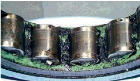
Lubricant degradation caused by electrical discharge currents
