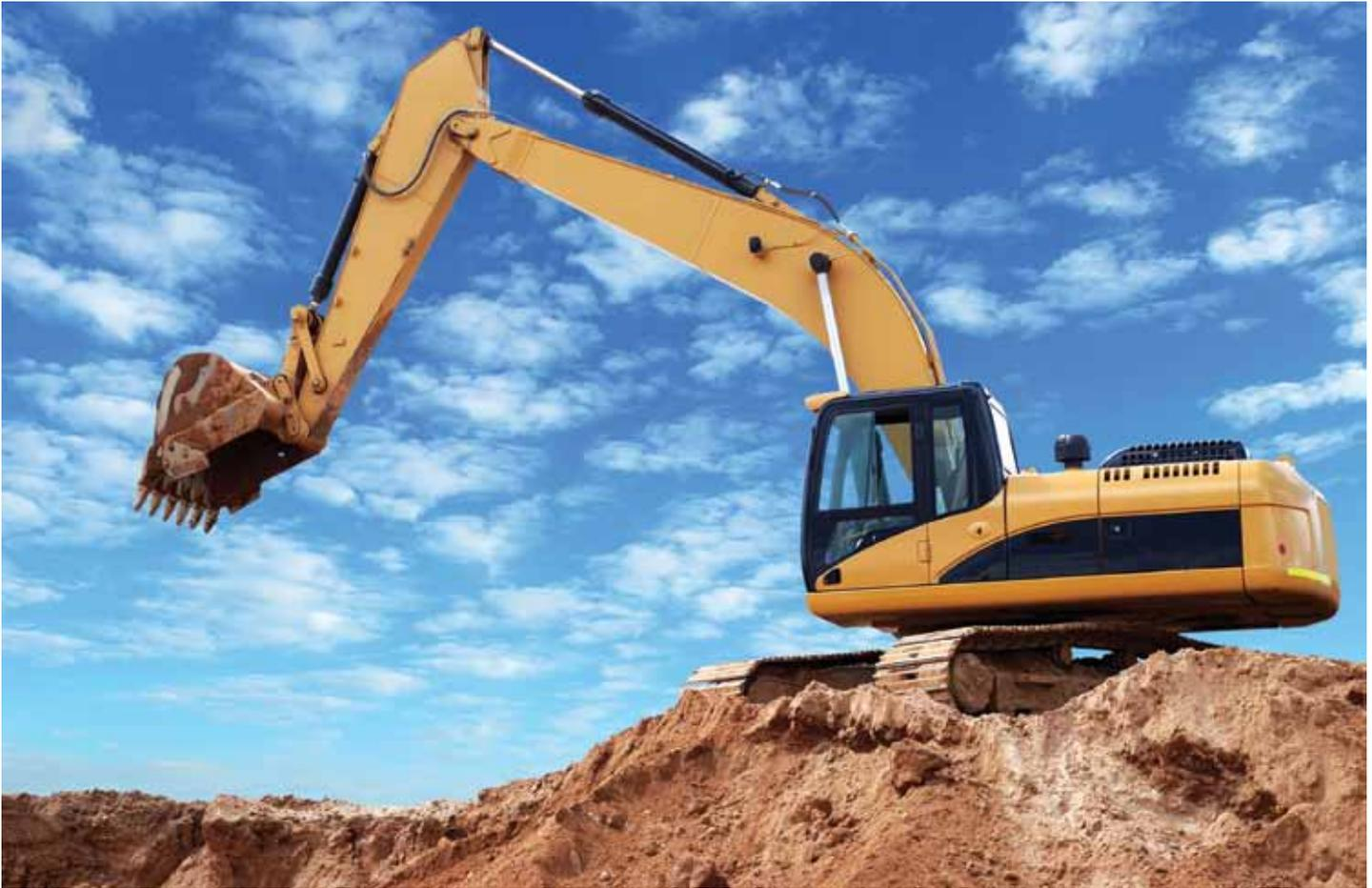
Monitoring engine loading and hydraulic pressure allows the control system to improve digging productivity while working to optimize fuel consumption.
