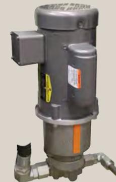
The DFC utilizes an industrial rated motor and a Parker H series fixed displacement loaded gear pump which has a high tolerance to system contamination.
