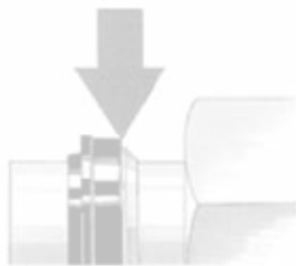
Fig. T50 — Ferrule cocked on tube
