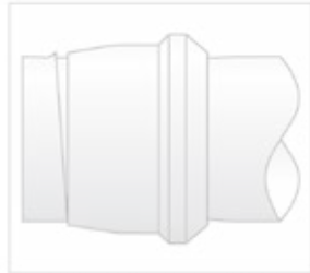
Fig. T50 — Ferrule cocked on tube
