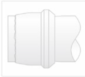
Fig. T47 — Tube not bottomed
