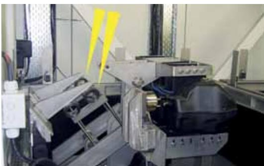
ACE-TUBUS bumpers are the alternative for applications in which the mass does not have to be stopped in an exact position or the energy does not have to be 100% removed.
