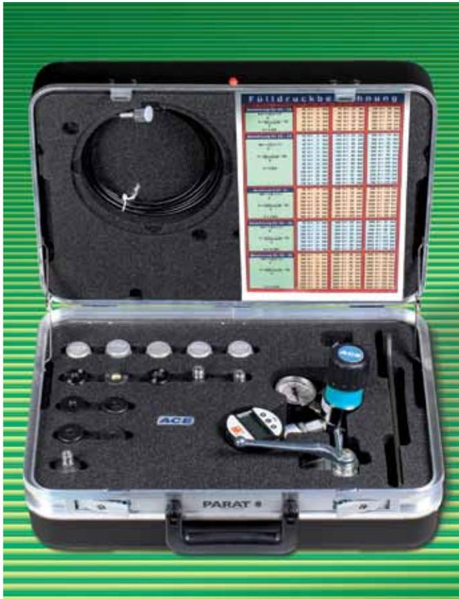
The **ACE gas spring refilling kit** offers you the opportunity to fill gas springs on location or adapt them individually. The refilling kit is equipped with all the parts you need to fill gas springs. Very precise filling of the gas springs is possible using the digital manometer. The table for determining the filling pressure of the gas springs is included with the case. The only thing missing from the delivery is the nitrogen.
