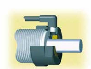
By using the air bleed adaptor the operating lifetime of shock absorbers in aggressive environments can be considerably increased. The adaptor protects the shock absorber seals from cutting fluids, cleaning agents, cooking oil, etc. by using a low pressure air bleed.
