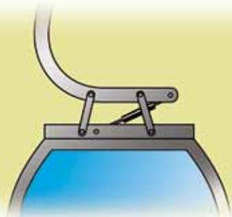
**Swinging movements cushioned by hydraulic dampers**
