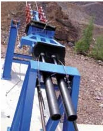
ACE safety shock absorbers are designed for emergency-stop situations in industrial and crane applications. They are individually tailored to the relevant application for emergency-stop.
