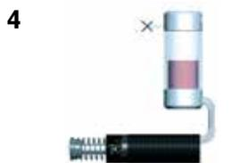
Spring return with air/oil tank. No air supply connected. Note: Will extend return time.
