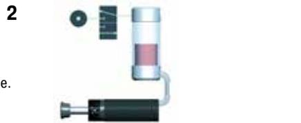
Return stroke may be sequenced by pneumatic return valve at any desired time. No return force until valve energized.
