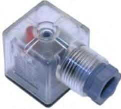
Solenoid Valve Connector, Field Wireable, 3 Pole, Form A 18mm, 10A, LED w/MOV, PG9 opening
